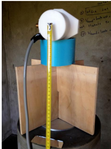
Photograph showing the proton bottle on a support 35 cm above the pillar.
