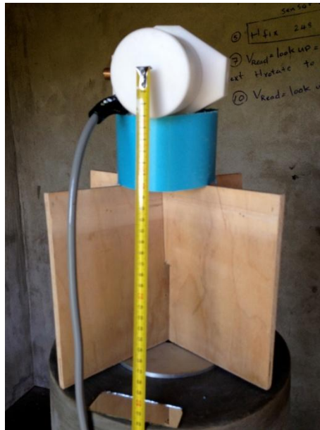
Photograph showing the proton bottle on a support 32.5 cm above the pillar.
